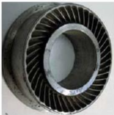
Exhibit 2 depicts the aircraft engine metal part, ECM machined.
